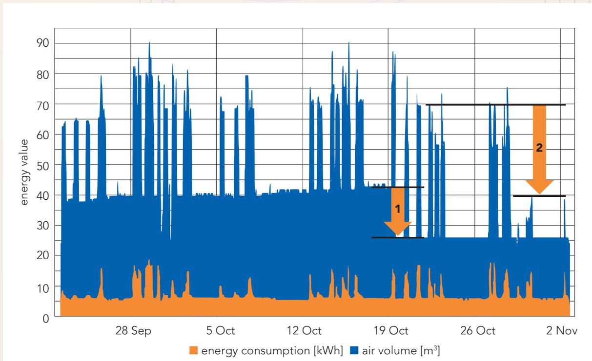
Figure 16: Extract from the operating status report to indicate the required air volume before and after an event on a machine. (Source: INNIO Jenbacher)
