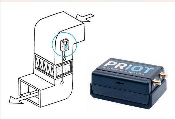
Figure 3: IoT sensor to be installed at the filter system. (Source: [www.priot.ch](http://www.priot.ch))
