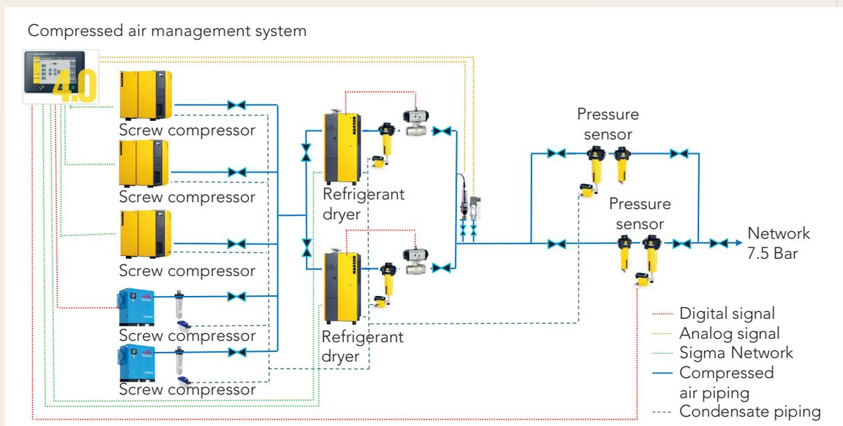
Figure 11: Simplified schematic.
