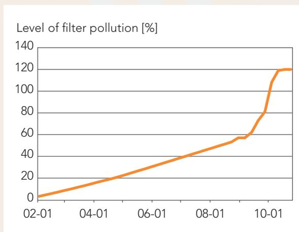
Figure 5: Evolution of filter pollution according to measured data of the IoT Sensor. (Source: PRiOT)
