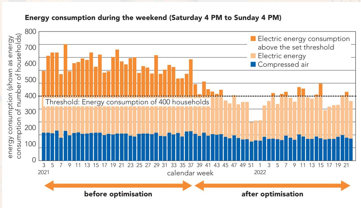
Figure 15: Electricity (light and dark orange) and compressed air (blue) consumption on weekends before and after project (shown as energy consumption of number of households). The dotted line shows the defined threshold. (Source: INNIO Jenbacher)
