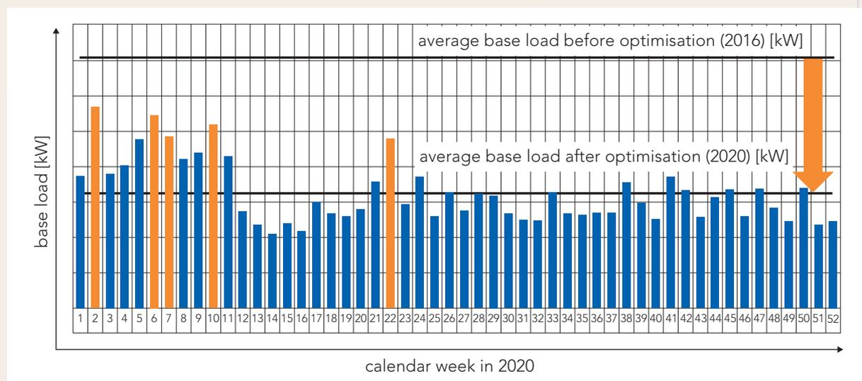
Figure 13: Illustration of the base load values of the crankshaft lines per calendar week in 2020. Orange bars represent the exceedances of the base load target values on the respective weekend.
