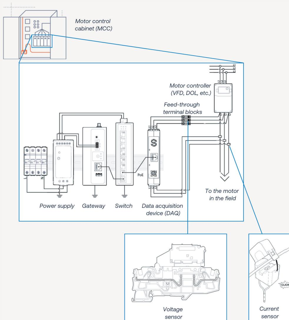
Figure 2: Electrical signature analysis sensors attached to the electrical wires in the motor control cabinet.
