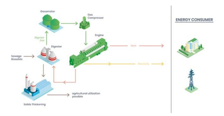
As a WWTP operator, you can capitalize on the power you produce with CHP and use it as a reliable, independent supply for your wastewater treatment. Waste heat from combustion processes can be used to heat up the biosolids in the digester and thus heat your entire plant.
